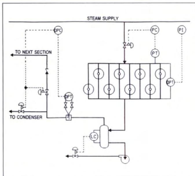
Figure 3: Blow-through for cascade system
