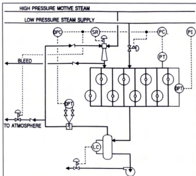
**Figure 2: Blow-through with thermocompressor.**
